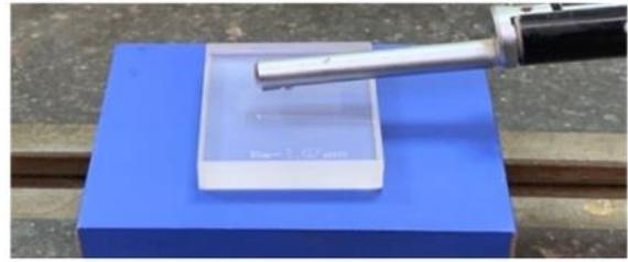
Fig. 8 Calibration of the profilometer by using 1.64  $\mu\text{m}$  block
