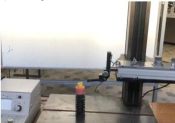
Fig. 6 Taylor Hobson Roughness Profilometer device and Ra reader
