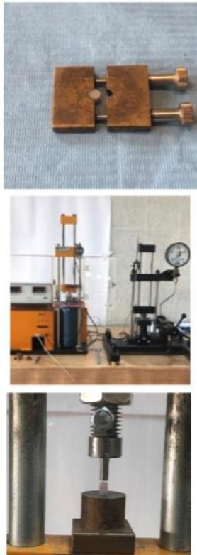
Fig. 9 Compressive strength test procedure: (A) Cylindrical metal mold filled with tested materials, (B) Specimen of 4.0 mm diameter and 6.0 mm height, (C) Universal testing machine, (D) Specimen before load application
