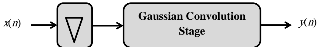
Fig. (6): A 1 st order derivative Gaussian system model (using Gaussian function and a derivative stage).
